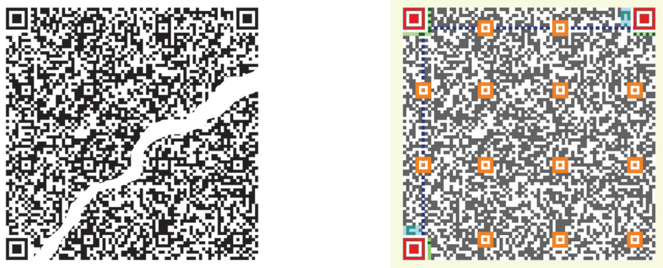
Figure 2. QR code structure and tolerance. Left: QR code with the maximum level of error correction (H: 30% of tolerance to damage). Right: Structure of the same QR code: yellow: quiet zone; red: position; orange: alignment; blue: timing; green: format information; cyan: version; grey and white: data and error correction modules.
